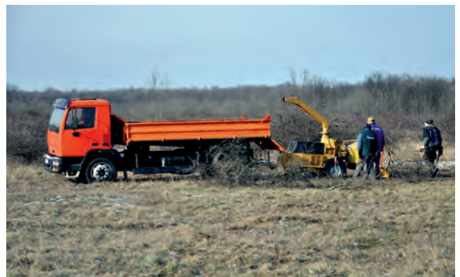
Fig. 6. The eradication of invasive woody species results in woody plant parts. A woodchipper is often used for reducing these parts into smaller woodchips. (Photo: M. Korda)
