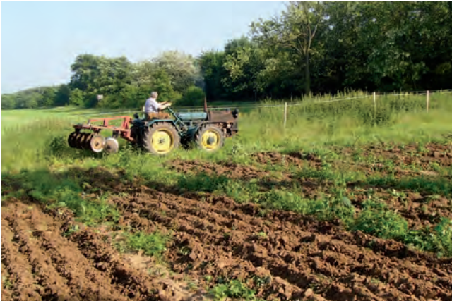
Fig. 7. Soil cultivation with disc cultivator attached to narrow-gauge agricultural prime mover. (Photo: A. Csór)
